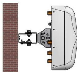
Note: If the bracket is used in applications that provide additional tilt to the antenna (e.g. slanted poles, upside down hanging, etc.), different weep holes may be required. Please consult our weep hole guide at [jmawireless.com/support](http://jmawireless.com/support).
