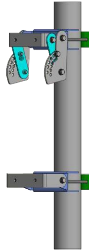
JMA PART # 919017 2 POINT, 0-22 DEG DOWNTILT 3.5" MAX POLE SIZE
