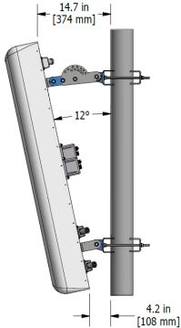
CSS P/N: 919036 BRACKET KIT 2 POINT, 12 DEGREE DOWN TILT SHOWN MOUNTED ON 4.5" O.D. POLE 4.5" O.D. MAX POLE SIZE
