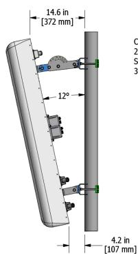
CSS P/N: 919011 BRACKET KIT 2 POINT, 12 DEGREE DOWN TILT SHOWN MOUNTED ON 3.5" O.D. POLE 3.5" O.D. MAX POLE SIZE
