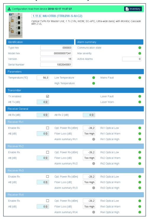
The **MU-OTRX (TTRU2W-S-M-C2)** panel includes the following information about the selected plug-in optical module for DAS designs delivering seven or nine bands on a single fiber:
