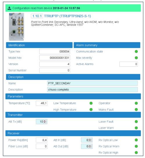
The **TTRUPTP Secondary without 4-way splitter/combiner** panel includes the following information about the secondary Point-to-Point module, without four-way splitter/combiner module:
