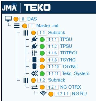
Each node in the **Physical Tree** is associated with an icon and an ID number. The icon identifies the component type; the ID number represents the component position in the DAS. See "[Viewing the System Architecture](#)" on page 18 for a detailed description of the **Physical Tree** device hierarchy.
