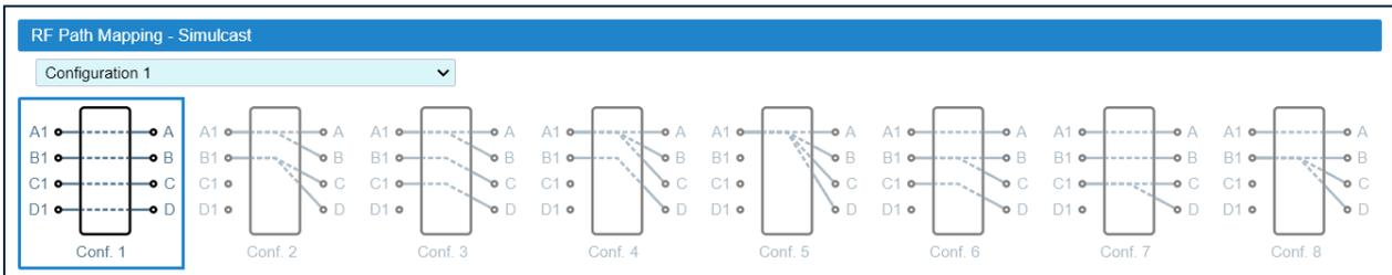
*Configuration 1* is the default factory configuration. When you select a configuration from the drop-down list, the diagram that corresponds to the selected configuration is highlighted. You can choose between eight different simulcast configurations.
