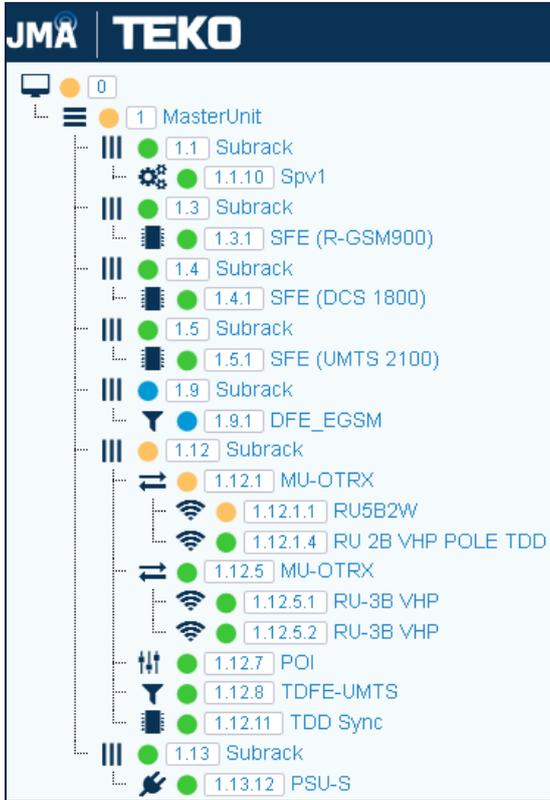
In the **Physical Tree**, each node is associated with an icon and an ID number. The icon identifies the component type; the ID number represents the component position in the System. See "Device Hierarchy" on the next page for details.
