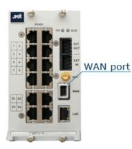
**Caution:** Never connect the Wide Area Network to the LAN port. The DHCP server, running on the LAN port, may cause connectivity issues in the Wide Area Network.
