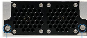
Captive screws (M4x18) fastening the fan unit to the sub-rack
