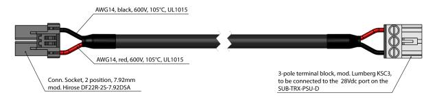
**Note:** The following figure shows an additional power supply cord that is provided with each SUB-TRX-PSU-D sub-rack. Use this cord only if power supply connections between two SUB-TRX-PSU-D sub-racks are necessary:
