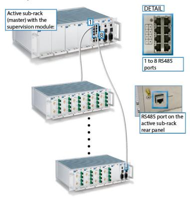
**Note:** If ports S1 to S4 are not connected to remote Point-to-Point components, they can be used to manage additional sub-racks installed at the master unit site.
