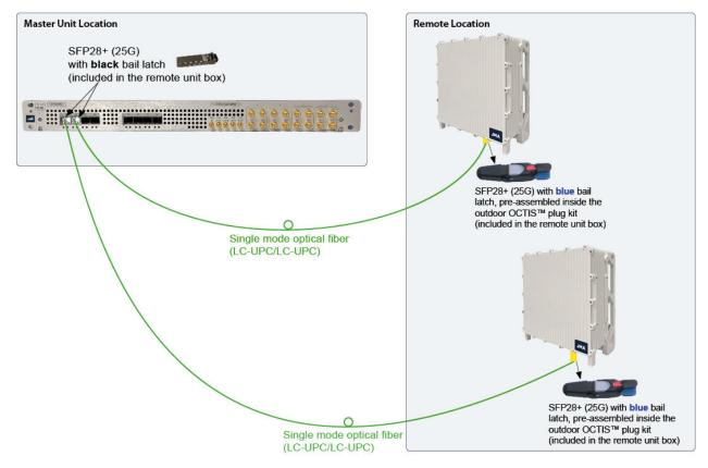
Connect the optical cable from the remote unit to the optical port on next generation optical transceiver as described in the following steps:
