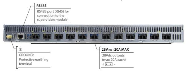
Each Vdc output connector is protected by a fuse. If a fuse blows, the green LED next to the connector switches off and the output voltage alarm for the connector is triggered (See the *JMA DAS Platform Troubleshooting Charts*).
