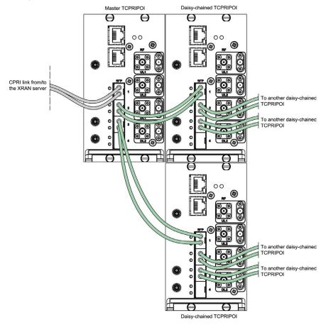
Up to two daisy-chained TCPRIPOI units are supported for each TCPRIPOI.
