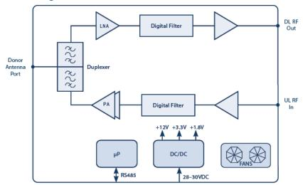
Each TDFE module hosts the duplexer, to be connected to the Donor Antenna to separate/combine downlink and uplink paths. In downlink the signal from the Donor Antenna is preamplified by a Low Noise Amplifier and converted into an IF signal by a down converter. The selection of the band of frequencies or channels to be extended is handled by a digital filter.
