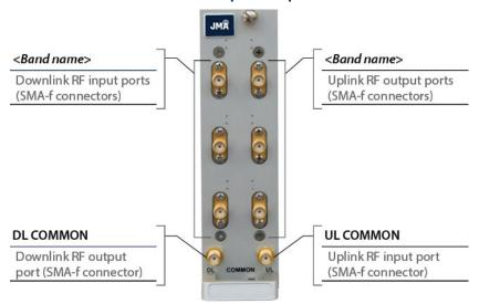
Triplexers (FDD) with Built-in 1:4 Splitter/Combiner TRI-SC4W-x - Input/Output Ports
