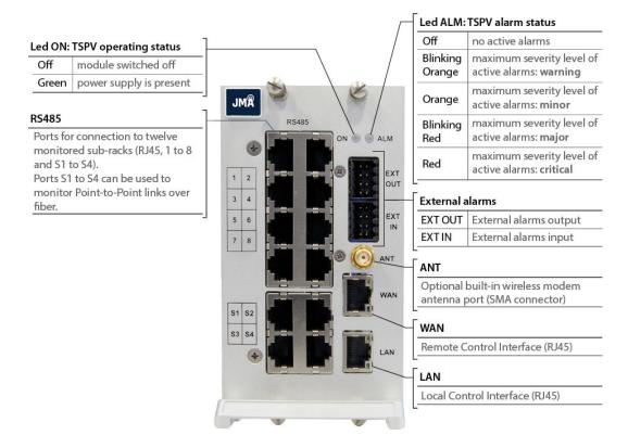
When all 12 front ports are connected to monitored devices, an additional power supply unit (SUB-PSUN-MU or SUB-PSUN-MU/48) can be monitored through the RS485 (RJ45) rear port of the sub-rack that hosts the supervision module. See "Connecting RS485 Communication Cables" on page 74.
