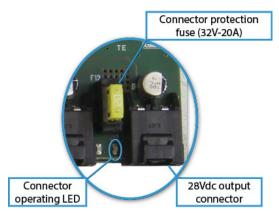
**Note:** To disconnect a power cable, first press the connector release tab, then pull the cable out.
