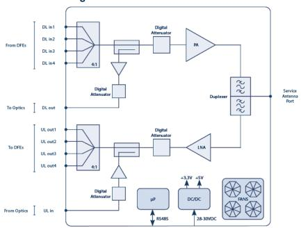
The TSFE hosts the duplexer, to be connected to the Service Antenna to separate or combine downlink and uplink paths. In the downlink, the signals from the Donor Front-End Modules are combined and amplified by a Power Amplifier. In the uplink, the RF signal from the Service antenna is amplified by a Low Noise Amplifier (LNA) and split to feed up to four Donor Front-End modules.
