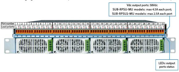
There are 32 LED indicators on the front panel of the PDU that show the status of each output port, as described in the following table:
