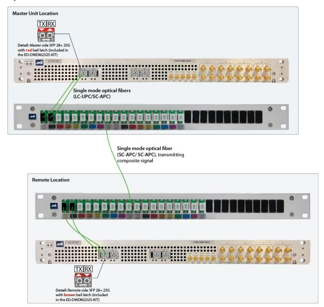
1. Insert the SFP+ with the **red** bail latch into the **ED35TDM** optical port (master side) and the SFP+ with the **brown** bail latch into the **ED35TDS** optical port (remote side).
