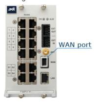
**Caution:** Never connect the Wide Area Network to the LAN port. The DHCP server, running on the LAN port, may cause connectivity issues in the Wide Area Network.
