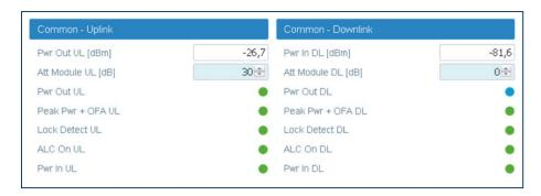
After successful completion of relevant training courses, use the commissioning tool spreadsheet, provide by JMA, to calculate uplink and downlink attenuation to be set.
