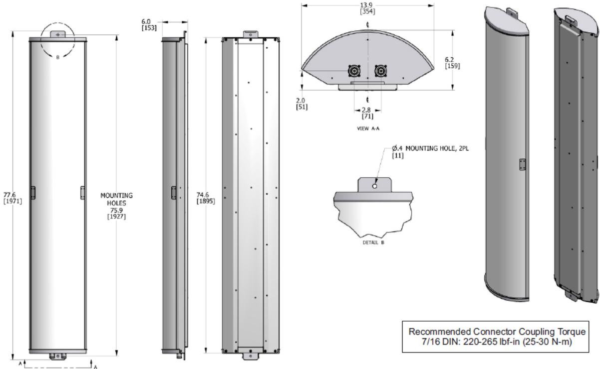
Recommended Connector Coupling Torque
