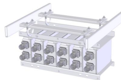
Ladder rack (front panel removed)
