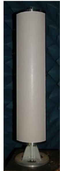
Single unit antenna shown specify electrical tilt of each unit (3 single units create the cylinder)
