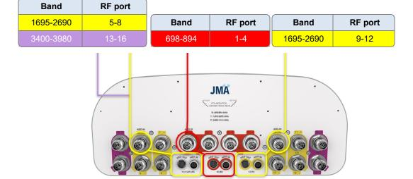
Note: The RET Device for 3400-3980 MHz is connected via the 1695-2690 Port 5 Bias T port or 1695-2690/3400-3980 MHz AISG ports.
