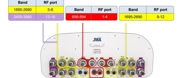
Note: The RET Device for 3400-3800 MHz is connected via the 1695-2690 Port 5 Bias T port or 1695-2690/3400-3800 MHz AISG ports.
