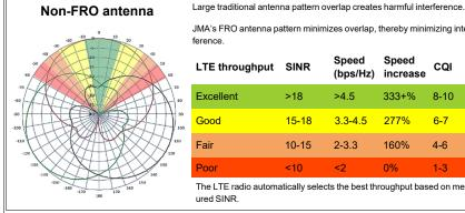
JMA's FRO antenna pattern minimizes overlap, thereby minimizing interference
