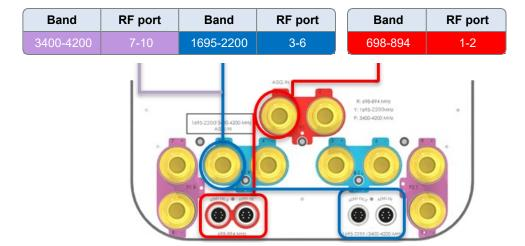
Note: The RET Device for 3400-4200 MHz is connected via the 1695-2200 Port 3 Bias T port or 1695-2200/3400-4200 MHz AISG ports.
