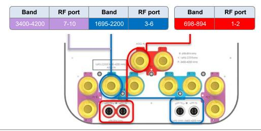
Note: The RET Device for 3400-4200 MHz is connected via the 1695-2200 Port 3 Bias T port or 1695-2200/3400-4200 MHz AISG ports.
