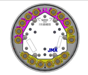
End view details: 6 stud bolts for direct mount to the Universal Sleeve (SC-BKT-SLA)
