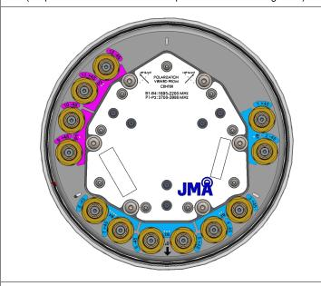
End view details: 6 stud bolts for direct mount to the Universal Sleeve (SC-BKT-SLA)
