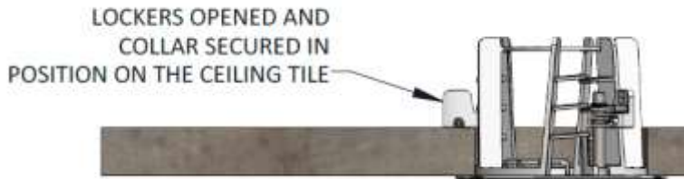
Figure 3: Screwing the lockers open
