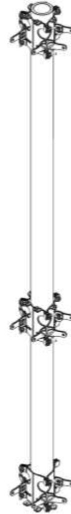
Figure 4: Brackets on pole (8' model for example)
