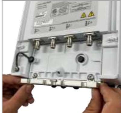
Step 2: Insert bracket tabs between plastic washer and captive screw head.
