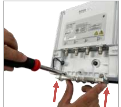
Step 3: Apply upward pressure on bracket while installing. Tighten both captive screws until complete resistance and torque per manufacturer's specification.
