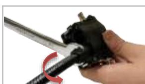
To remove the connector, rotate the Cap-Seal a quarter turn counter-clockwise and pull.
