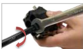
Rotate the Cap-Seal a quarter turn clockwise in the housing to secure the connector in place. A 14mm or 9/16in wrench may be used in confined spaces.
