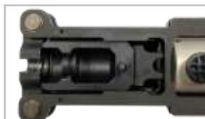
Insert the INSERTK into the frameset so the narrow side is oriented toward the cable opening.
