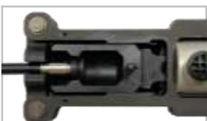
Pull/push back the frameset to allow connector/cable to lie flat in the frame.
