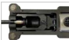
Make sure connector is fully seated. Press HCG trigger until compression tool cycles. Do not pull or push on tool during compression.
