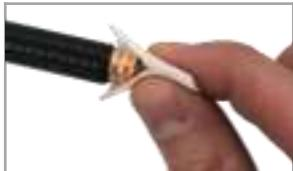
Use the alcohol wipe to clean the inner and outer conductors thoroughly.
