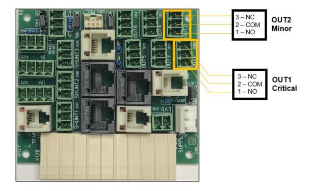
Board is on rear of rack behind Orion controller (interface connectors are included with unit).
