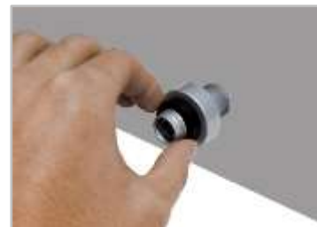
Install port seal, with text "This side away from nut" toward port. Seal is black in color.
