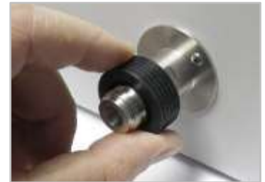
Install port seal, with text "This side toward nut" facing nut. Seal is black in color.
