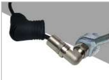
Torque the connector to 8 lbf-ft using the TQ-78-F8 torque wrench.
