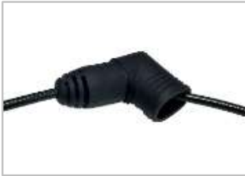
Slide the WPS-NRA-1S boot onto the 1/4" cable 8-12" from the end prior to cable prep.
