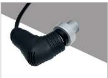
Slide the WPS-NRA-1S over the elbow and onto the port seal until ribs are no longer visible.
