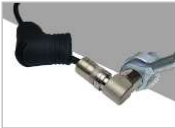
Torque the connector to 14 lbf-in using the TW1412 torque wrench.
