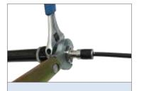
When using the torque wrench, make sure the mating connector is supported by an adjustable wrench.
