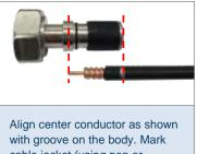
cable jacket (using pen or marker) in line with end of connector.
