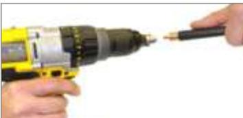
Use the coring bit "U" to remove dielectric until cable reaches stop on tool. You may optionally use the included T-Handle to prep/strip and core cable.
