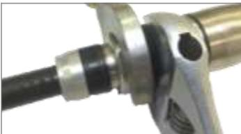
When using the torque wrench, make sure the mating connector is supported by an adjustable wrench.
