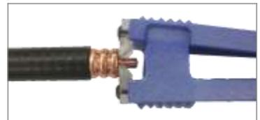
Use center conductor cleaner ("SP-CC tool") to remove any remaining dielectric material on center conductor.
