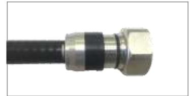
Push connector onto cable until it reaches alignment mark (until 2 clicks are heard/felt).
