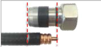
Align outer conductor as shown with o-ring on body. Mark cable jacket (using pen or marker) in line with end of connector.
