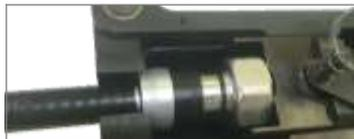
Pull/push back the insert to allow connector/cable to lay flat in frame. Make sure connector is fully seated. Press HCG tool trigger until gun cycles. Do not pull or push on tool during compression.
