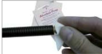
Use alcohol wipe to clean inner and outer conductors thoroughly.
