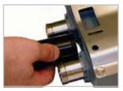
Measure the WPS-DF from the end of the port to the beginning of the threads shown. Use your thumb to mark a cut line.
