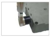
Torque the connection to 18 lbf·ft using the TQ-114-F18.
