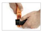
Align the blade of the RDCUTTER to the thumb mark indicating the cut length. Using one firm cutting motion, cut the WPS-DF to the proper length.
