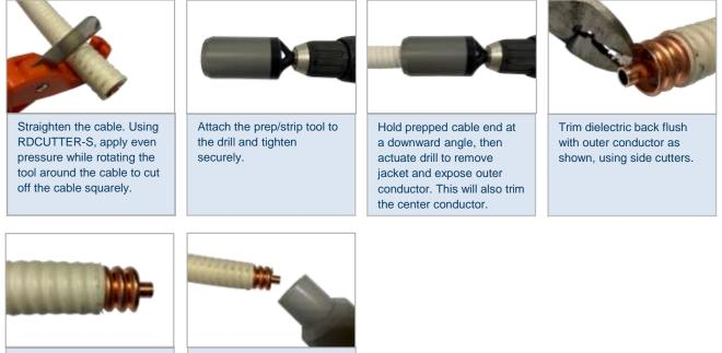
Properly stripped and prepped cable is ready to be vacuumed to remove residual dielectric and
