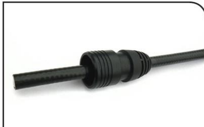
Prior to cable preparation, slide the WPS-4A or WPS-4S onto the 1/2" cable 6-12 inches from the end.
